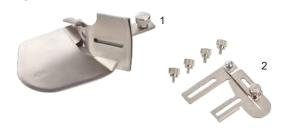
With the single fold binder attachment, fabric edges and necklines can be perfectly bordered with bias tape. The unfolded tape is inserted through the attached guide rail, folded over on the upper side while the under side remains open, and is then sewn on with a cover stitch. For the perfect look, the bias tape can also be self-made.
